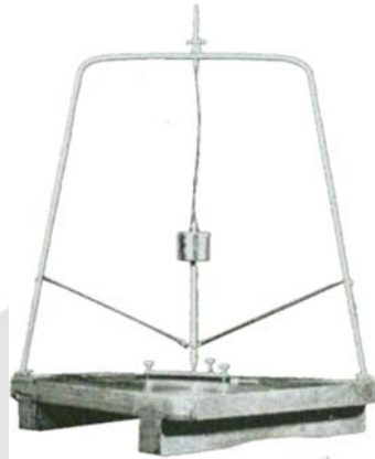
Figure 2-9 Reconstruction design of Zhang Heng's seismoscope by A. Imamura (1939) [09]
