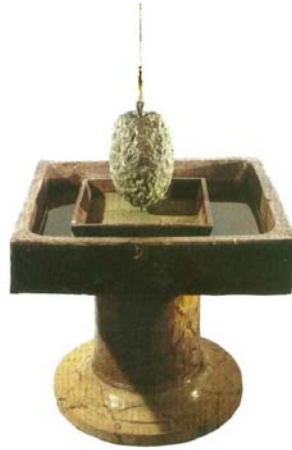
Figure 4-5 Andrea Bina's seismoscope [37]
